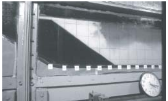
Figure 3 Establishment of a delta composed solely of black sand in Experiment 1. The flow is from left to right. The squares on the glass wall of the flume, which are 10\text{ cm}^2 , provide scale for this and other figures below.
