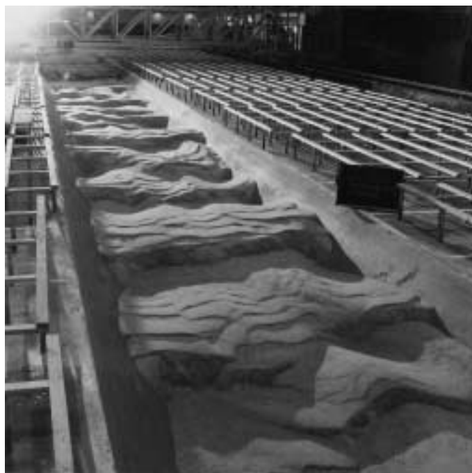
Fig 3. Bedform patterns for relative depth of 0.3
