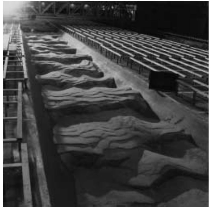
Fig. 3. Sand dunes for low overbank flow with rough floodplains, Q = 0.350\text{m}^3\text{s}^{-3}
