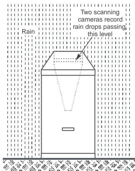
Fig. 1. 2-D Video disdrometer: sensor unit containing cameras and light sources.
