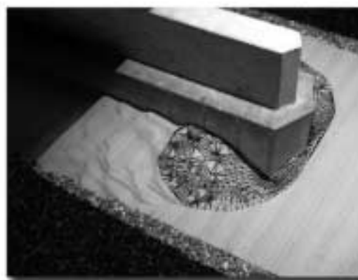
b. Triangulation mesh overlaid with side view
