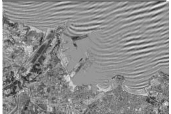
Fig. 1 A snap shot of the free surface elevation based on the numerical simulations of wave propagation near Gijon Harbor (Spain), using a parabolic approximation of the mild slope equation for spectral wave conditions. (GIOC, 2000).
