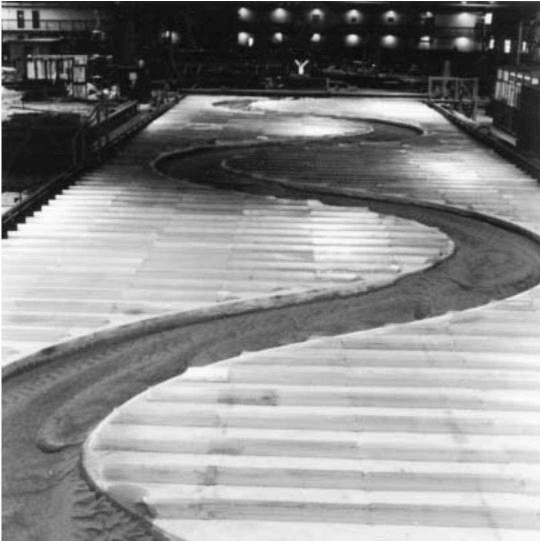
Fig. 2. View of UK Flood Channel Facility – Series C tests with metal floodplain roughness units in place.
