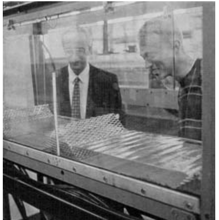
Fig. 4. View of tilting flume showing calibration tests on expanded metal roughness units in progress.
