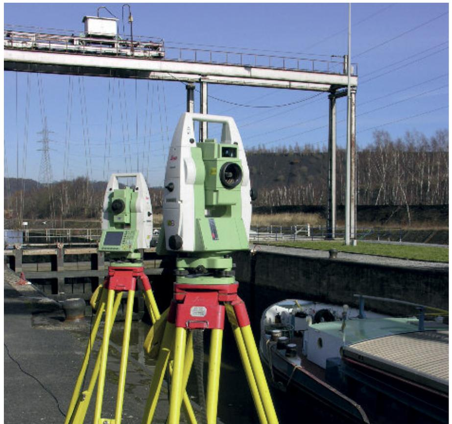
Figure 1. Measuring vessel position at Roselies lock
